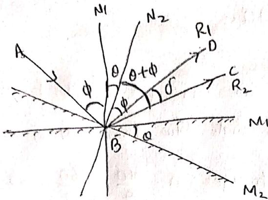
Here  $M_1$ ,  $N_1$  and  $R_1$  are the initial positions of mirror, Normal and direction of Reflected ray
