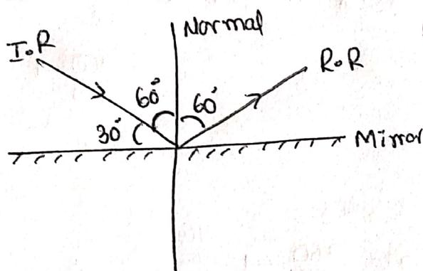
Angle of incidence is the angle between incident ray (I.R) and Normal to the plane mirror.
