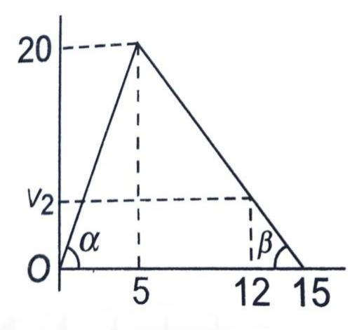
$$aneta = rac{v_2}{(15-12)} = rac{20}{(15-5)} \Rightarrow v_2 = 6m/s$$
