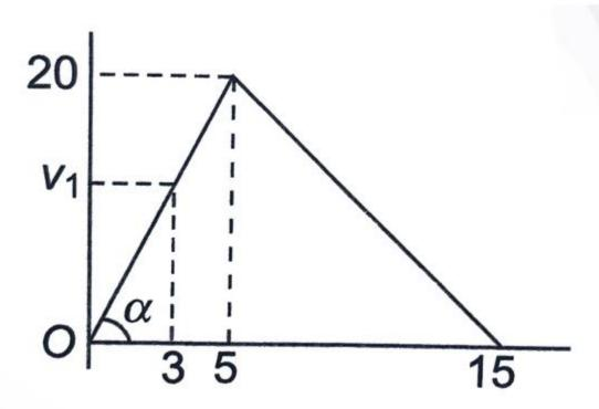
$$\tan \alpha = \frac{v_1}{} = \frac{20}{} \Rightarrow v_1 = 12m/s$$
